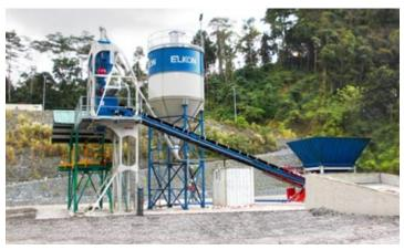
The weighing process of the aggregates is done for all aggregates consecutively while loading the materials from loader to the aggregate bunker. Also the loader operator can easily check the amount of aggregate in the bunker by the screen located near the aggregate bunker.
