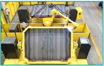
Using robotic welding technology has completely eliminated the negative effects of human factor in the production quality and increased the welding quality to excellent level. The production rate is also accelerated accordingly.
